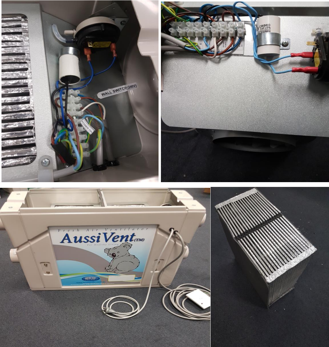
Illustration 12: Filter side power and wall controller connections for motor, and the H/X
